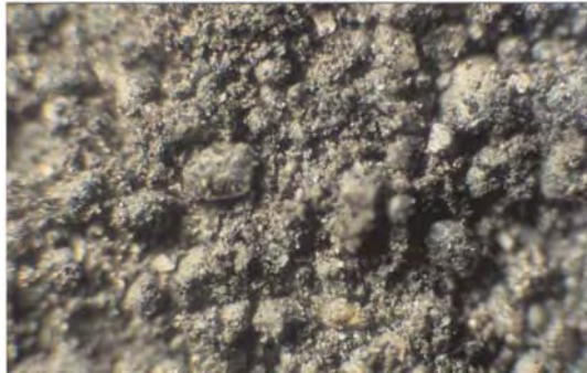
▲ Microscopic photo of residual foundry sand
